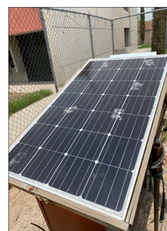
FIGURE 8. Monocrystalline photovoltaic panel.
