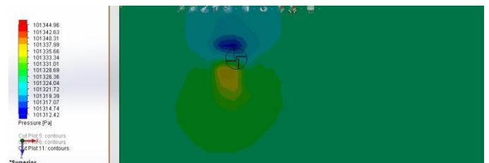
Figure 13 Pressure contour of the VAWT rotor
