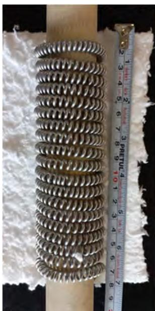
**FIGURE 2.** The heating element and its support. Heating element: electrical resistance wire (Length 11.1 m, diameter: 1.6 mm) based in Kanthal [12]. Support: Alumina pipe.
