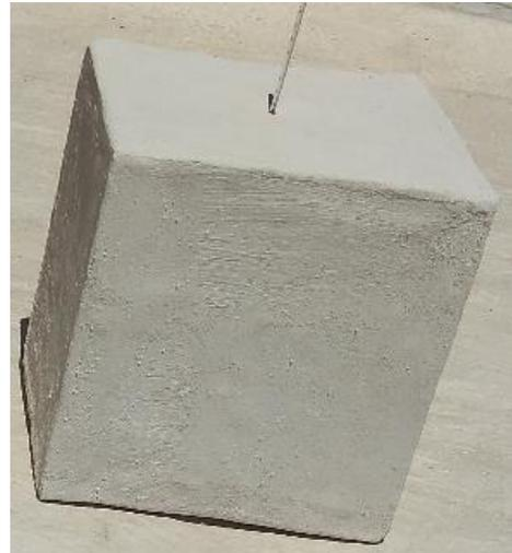
**FIGURE 3.** Box with a layer of plaster-polymer composite (PPC) to evaluate thermal performance in real sunny day conditions.
