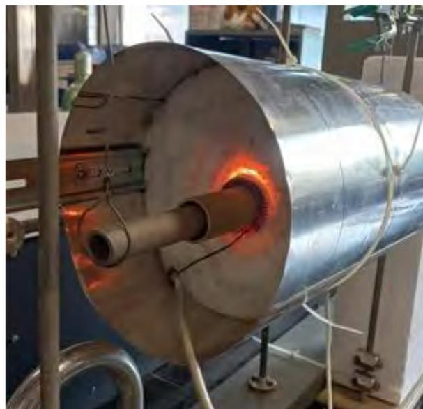
**FIGURE 1.** The apparatus. Thermochemical reactor consists of a steel tube (AISI 304). Two removable bronze – stainless steel heads for both the circulation of the reducing gas and the exchange of reactants and products. Thermocouples for measurement and control are K type, distributed throughout the body of the apparatus.
