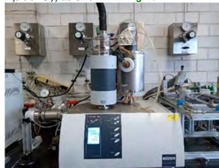
**FIGURE 7.-** NETZSCH unit model STA 449 F3 Jupiter assembled in the Solar Thermochemistry Laboratory UAM-I, Mexico.
