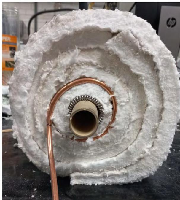
**FIGURE 3.** The heater and cooling coils surrounded by layers of thermal insulating material.
