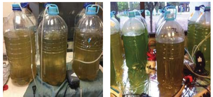
Figure 1, Growth Chlorella vulgaris in ARCV, ARCH and ARAR at environmental temperature ( 28\pm 2^\circ\text{C} ), photoperiod (day/night), aeration 1 vvm
