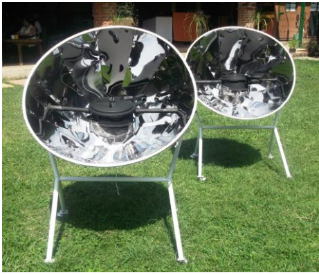
Fig. 3. The Rural Solar Cooker (RSC)
