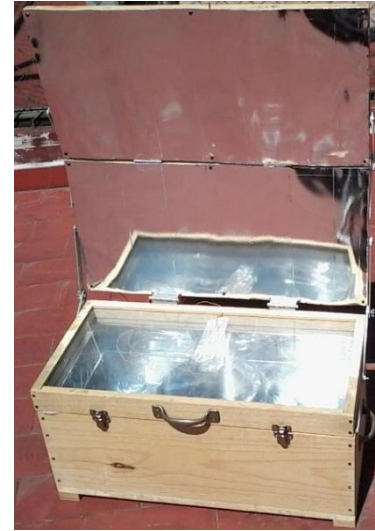
Fig. 1 Solar cooker box-type
